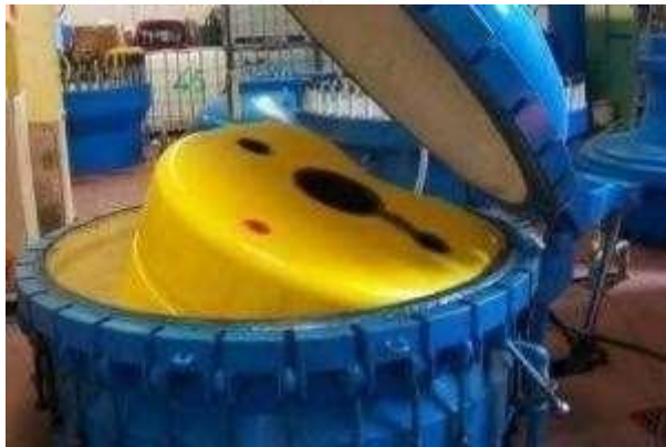
Hydrostatic pressure test
