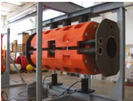
» Structural Pressure Test on the buoy body
