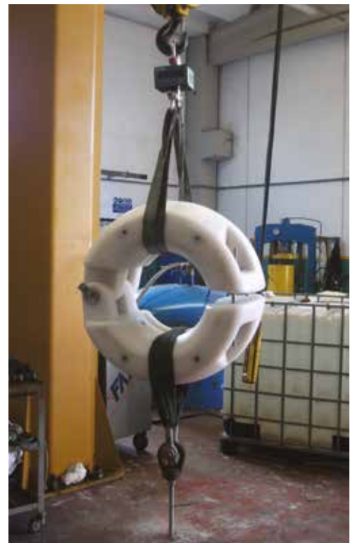
» Tension Test on float assembly
