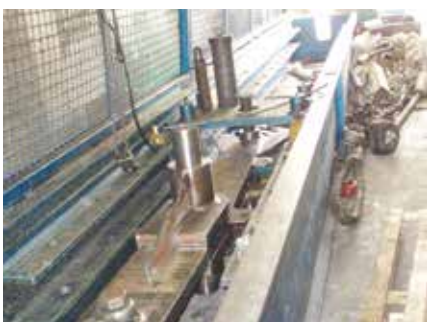
» Proof Load Test on steel parts
